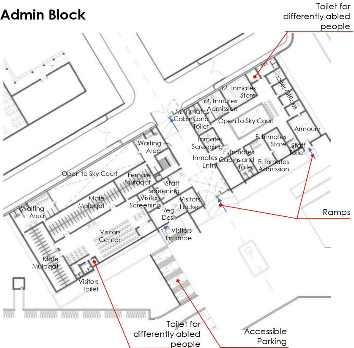
1. Handicapped Accessible Parking 2.7mx5.5m car park with 1.5m gap in between.
