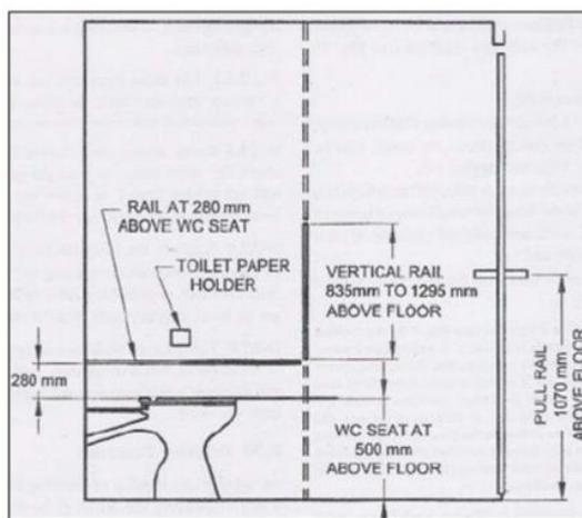
8. A unisex universally accessible toilet should be provided with minimum internal dimensions of 2200 X 2000 mm with an independent entry from the corridor and not from the single sex toilets. (Refer HGSS for details)
