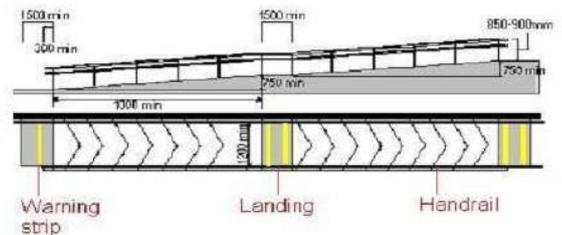
Fig. Landings and placement of tactile warning strips on a ramp
