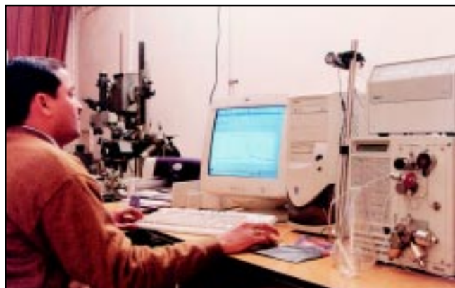
Analysis of High Explosive substance by High Pressure Liquid Chromatography system in CFSL (CBI), New Delhi
